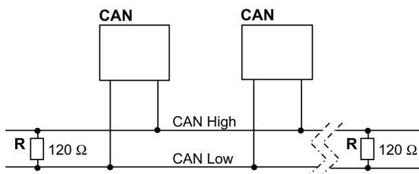
CAN CAN Bus device in actuator or other equipment
