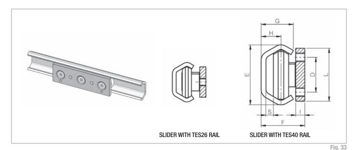
The sliders CES26 for the rail TES26 feature a zinc plated steel body with two fixing holes. With the rails TES40 can be used the sliders CEN40-135 indicated on page XR-10 that have a body with black color surface treatment.
