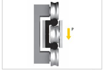
Composed of two FXRG rails with rollers in between the rails fixed to mobile part and rollers on fixed structure running on outer raceways, providing a customized solutions for telescopic movements.
