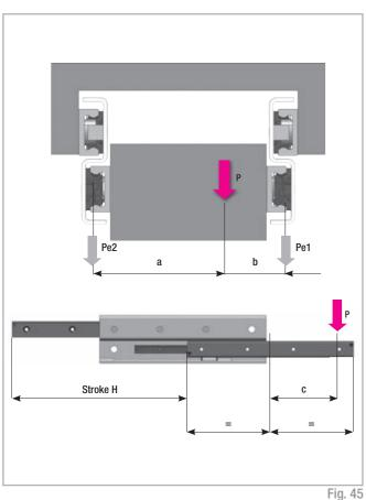
The main factors for sizing the slides for a telescopic movement:
