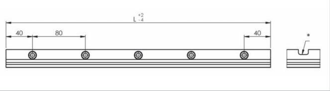
Fig. 15 \*Version FXRG-...-C with additional slot
