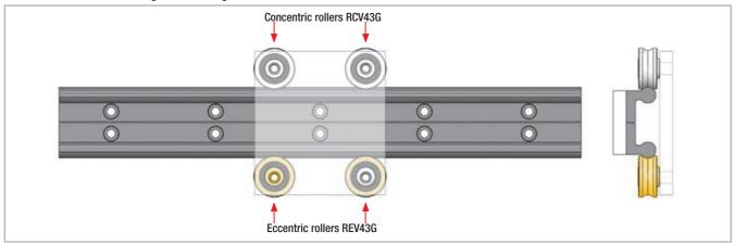
The rollers need to be positioned on the rail in numbers and directions according to the prevailing load. It is always preferable to orient the rollers so that the prevailing load acts radially, due to higher radial load capacity.
