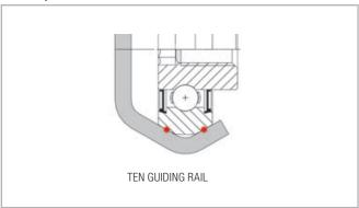
The two inclined bearing slopes run on the two slopes of the V-shaped raceways of the TEN rail. These 2 points contact on each roller in upper or lower raceway, assure both radial and axial load capacity.
