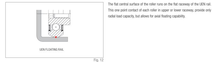
radial load capacity, but allows for axial floating capability.
