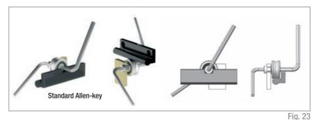
In case required to have eccentric rollers on the internal rail side, it is necessary to include optional accesses, to allow Allen-key to reach the roller. Otherwise the adjustment can take place outside of the rail.
