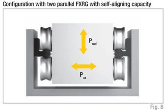
Configuration with two FXRG to form a single rail with a slider allowing for high Mx moments
